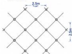
5 CABLE-NET GRID DETAIL SCALE 1:50
