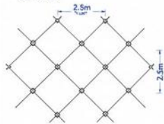
5 CABLE-NET GRID DETAIL SCALE 1:50
