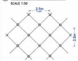
5 CABLE-NET GRID DETAIL
