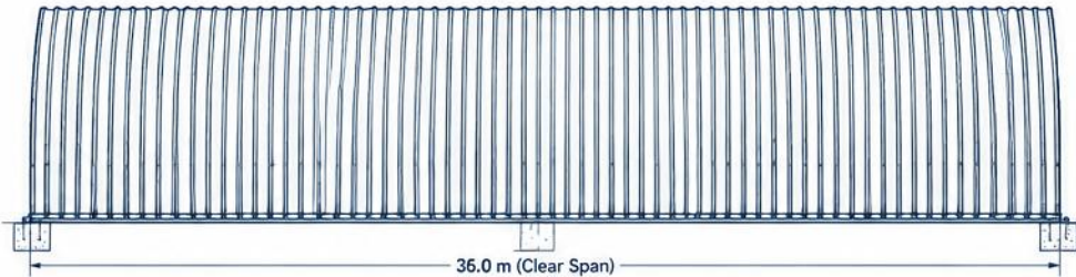
SIDE ELEVATION (Continuous Mechanical Seaming)
